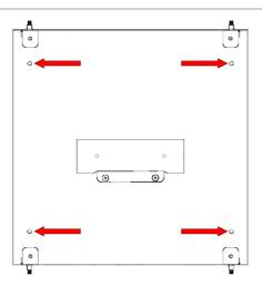
2. Secure cabinet to a wall using the 4 x Ø6mm holes as shown (fasteners not supplied).
