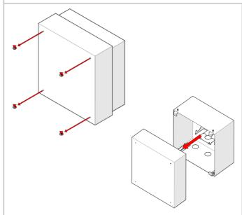
1. Measure & mark the cabinet mounting hole locations as per the *Dimensions* table. Remove the screws and front cover as shown.
