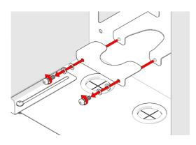
4. Remove screws, washers and valve bracket from the cabinet.
