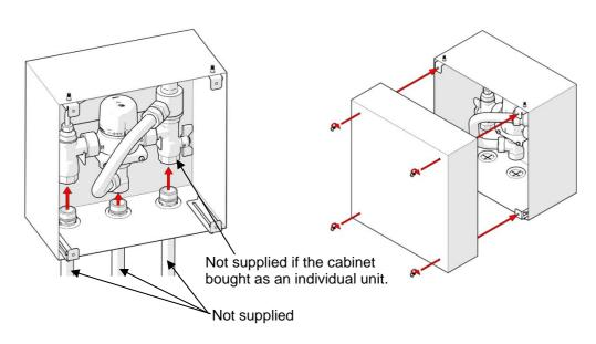
7. Connect inlets and outlet (not supplied with cabinet). Fit the front cover and screws.
