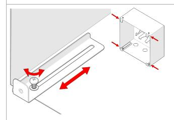
Adjust the front cover brackets on all 4 corners to the distance required. A minimum of approximately 60mm out is required for the valve to fit correctly.
